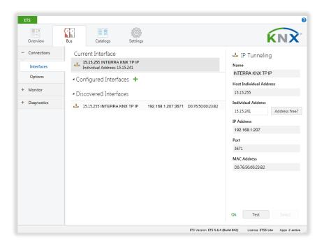
Fig 17: First Additional Physical Address (First Tunnelling Address) Assignment
