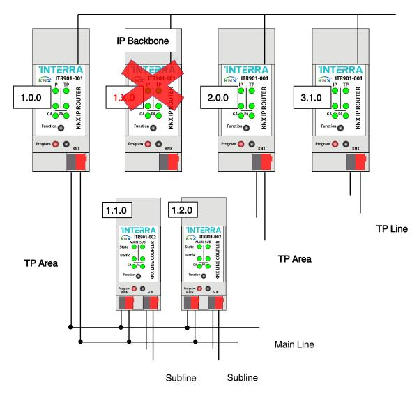
Fig 3: Interra KNX IP Router Network Topology
