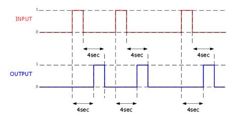
Fig 2. Switching Logic with 4 seconds delay
