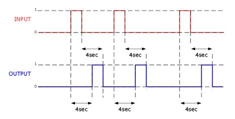
Fig 4. Toggle Logic 4 seconds delay
