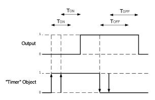
Fig5. ON/OFF Delays Retriggerable
