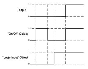
Fig8. AND Logic Function
