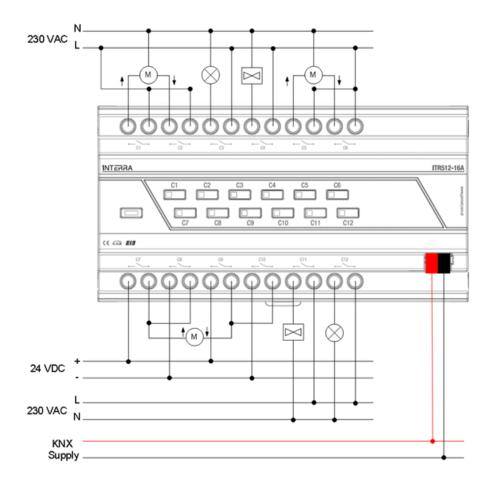
Fig23. Connection Diagram Example Configuration 3
