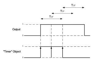
Fig3. Staircase Function Retriggerable
