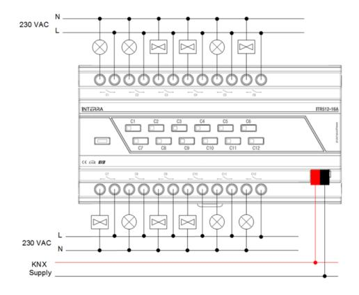
Fig21. Connection Diagram Example Configuration 1
