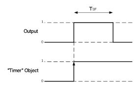
Fig2. Staircase Function
