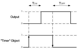
Fig4. ON/OFF Delays
