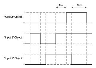
Fig1. Logic Gate with delays
