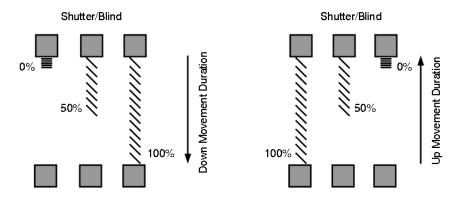
Fig19. Shutter/Blind Movement Duration
