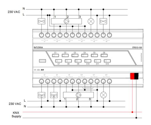
Fig22. Connection Diagram Example Configuration 2
